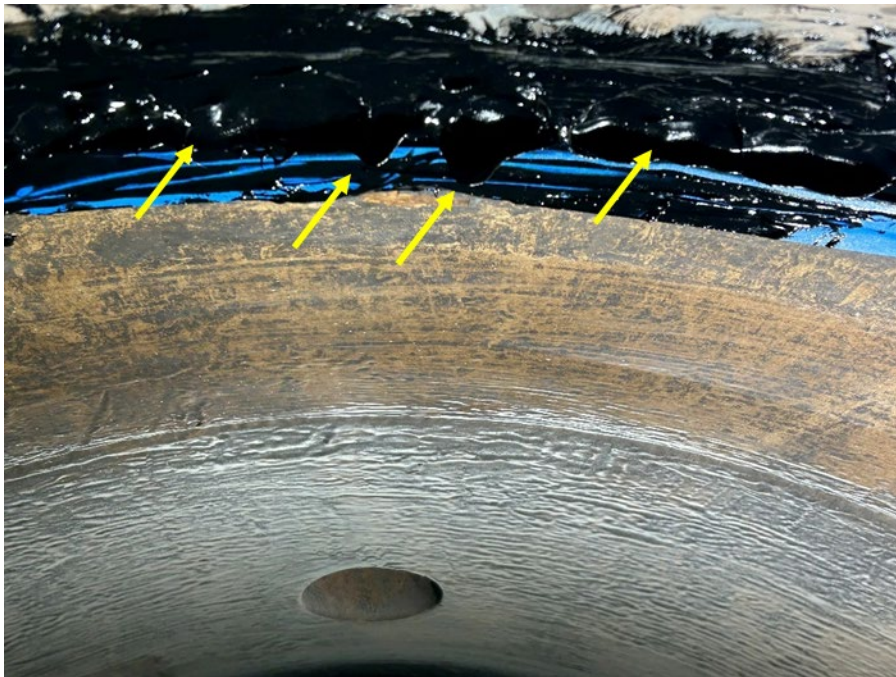
Figure 9.—PE2 is shown applied between the 11 o'clock and 1 o'clock positions. The lower viscosity resulted in sags and drips, noted with arrows.
